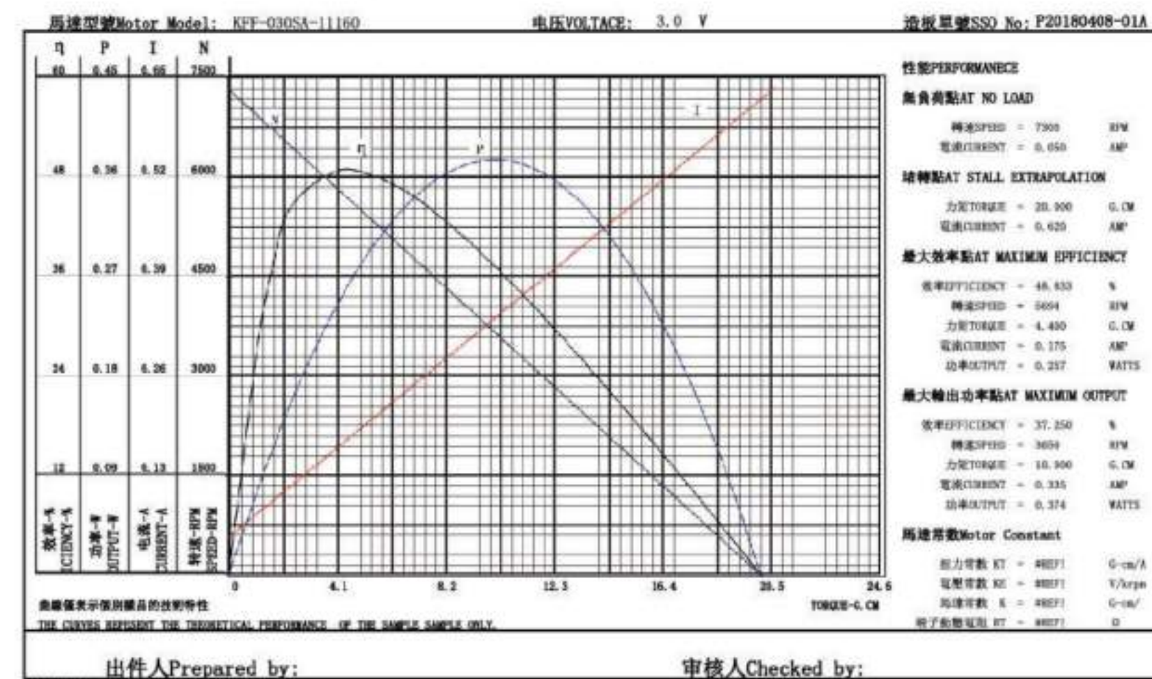
电机特性曲线 Motor Performance Curves and Characteristics
